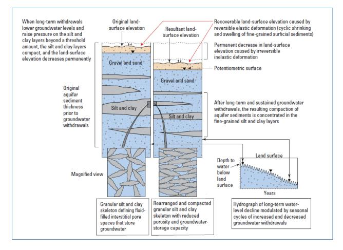
Figure 6-14. Mechanism of subsidence (from Kasmarek and others, 2015).
