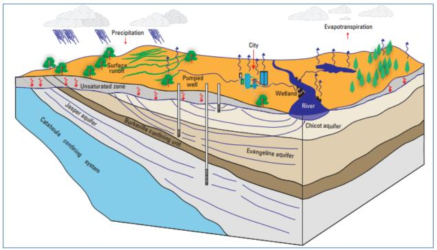
Figure 3-4. Conceptual model diagram of groundwater flow and the hydrologic cycle in Montgomery County (Oden and Delin, 2013).
