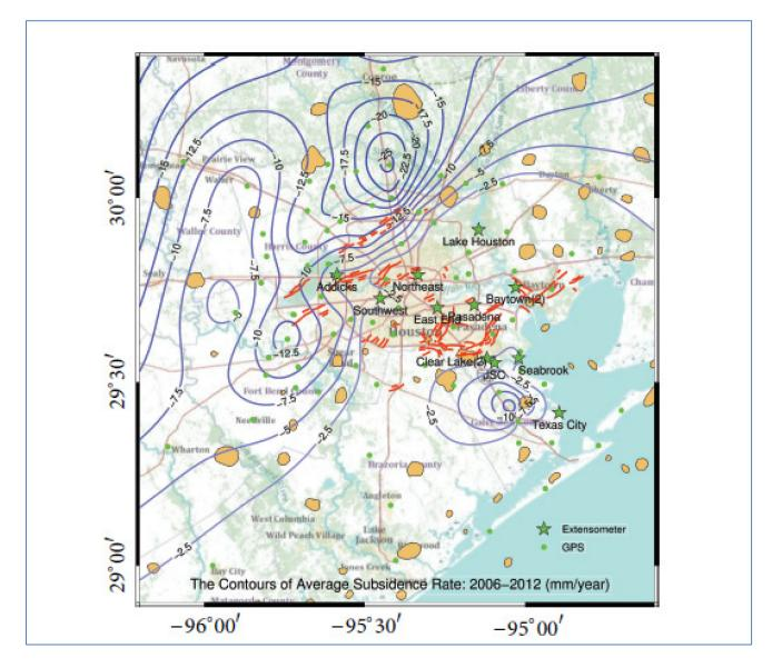
Figure 6-15. Map showing contours of the average subsidence rate, in millimeters per year, from 2006 to 2012. Red lines represent mapped faults and tan areas represent the locations of salt domes (from Yu and others, 2014).
