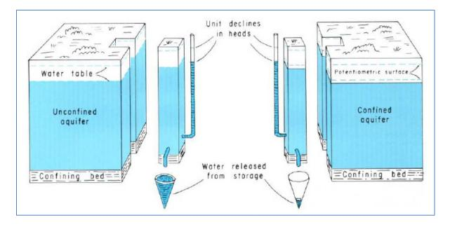
Figure 4-2. Differences in amounts of water released from storage in unconfined and confined aquifers (from Heath, 1983)
