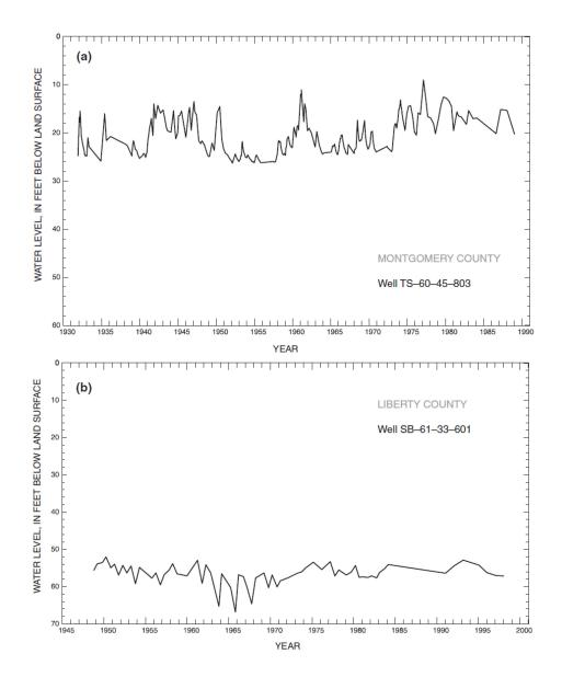
Figure 6-10. Hydrographs for outcrop area wells, showing relatively stable watertable elevations (Kasmarek and Robinson, 2004).
